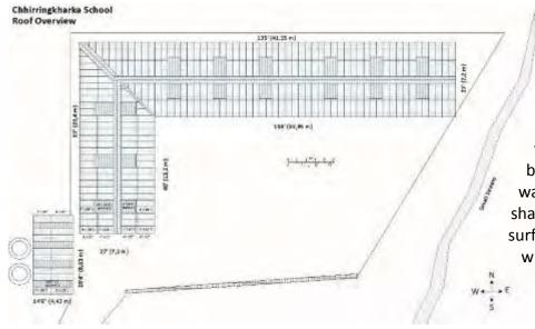
Roof Overview then you will have sufficient light from above in each classroom and in the toilet. There shall be taken very much care with the sheets when stored. It shall not be possible for people to walk on them, and they shall be placed on a level surface. The battens on which they shall be attached shall be in a completely straight line
